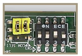
Ensure EVM configuration switch (SW3) are set as shown to run Power On Self Test (POST)
