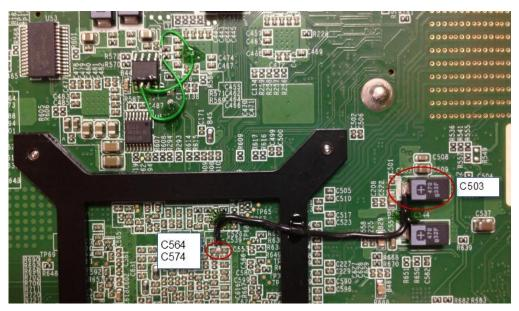
Note: That the rework should not link to GND and cause short circuit.
