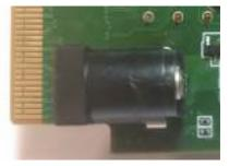
2. Move the COM1 to backside and adopt a 90 degree connector to avoid the interference with XDS560V2 mezzanine card.
